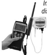
In order to compensate for any longterm drift of the transmitter, you can add an offset to the value displayed by the HTP300 with the EHK 500 reference portable instrument or via the keypad.
